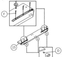
Step 6: Attach the drawer runners from pack 1 (6) to the drawer frame divider 1 (16) and drawer frame divider 2 (17) using hardware part F and a screwdriver (not provided). Insert hardware parts A and D using a small mallet (not provided).
