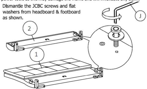
Step 17: Secure the headend (1) and footend (2) using hardware part J. DO NOT use any power tools as this may damage the frame and will invalidate any claim.
