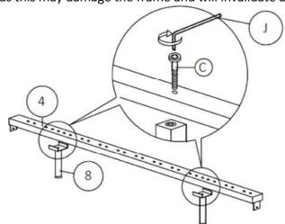
Step 19: Secure the centre rail into position using hardware part G and a screwdriver (not provided). DO NOT use any power tools as this may damage the frame and will invalidate any claim.
