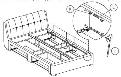
Step 21: Attach the slats (5) using hardware parts L and M, then secure the frame using hardware part J. DO NOT use any power tools as this may damage the frame and will invalidate any claim.
