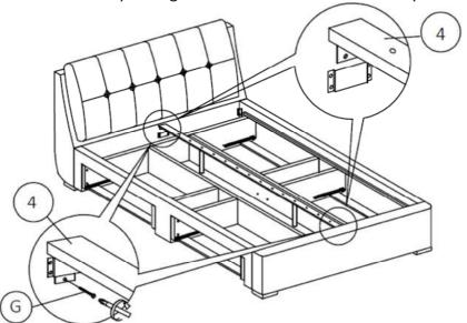
Step 20: Secure the frame using hardware parts C, J and K. DO NOT use any power tools as this may damage the frame and will invalidate any claim.
