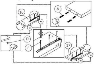
Step 7: Insert hardware parts A and D to the drawer frame crossbar (18) using a small mallet (not provided). DO NOT use any power tools as this may damage the frame and will invalidate any claim.
