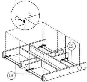
Step 13: Secure the frame using hardware parts B and J.
