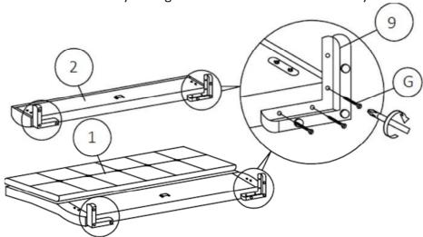
Step 16: Undo the screws and washers in the headend (1) and footend (2) using hardware part J. DO NOT use any power tools as this may damage the frame and will invalidate any claim.
