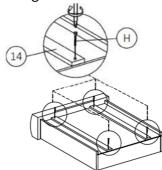
Step 4: Attach the drawer runners from pack 2 (7) using hardware part F and a screwdriver (not provided). DO NOT use any power tools as this may damage the frame and will invalidate any claim.
