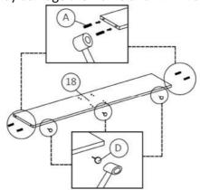
Step 8: Insert hardware parts A and D to the drawer frame crossbar (18) using a small mallet (not provided). DO NOT use any power tools as this may damage the frame and will invalidate any claim.
