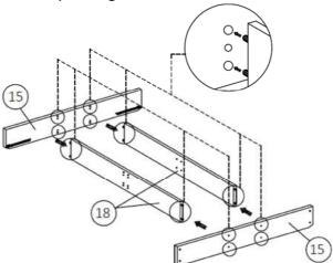
Step 10: Secure the frame using hardware parts B and J.
