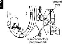
CONNECT THE WIRES. NOTE: Attach black fixture wire to black supply wire, white fixture wire to white supply wire. Do not mix them up. Use approved electrical tape or wire connectors (not provided). Connect bare fixture ground wire to ground wire from outlet box. NEVER CONNECT GROUND WIRE TO BLACK OR WHITE POWER SUPPLY WIRES.
