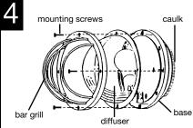
PLACE DIFFUSER ON FIXTURE BASE. Then place bar grill on frame over diffuser and attach to base with mounting screws (8-32 x 1/2, 4 combination head screws provided). NOTE: Outdoor wall fixture MUST be caulked with an acrylic caulk where base of fixture meets mounting surface. This provides a water tight seal when fixture is installed.
