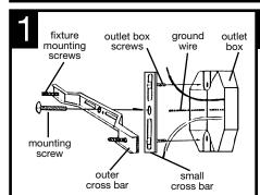
ATTACH small cross bar to outlet box with outlet box screws (8-32 x 1/2, screws not provided). THREAD fixture mounting screws (8-32 x 1,2 provided) into large cross bar.
