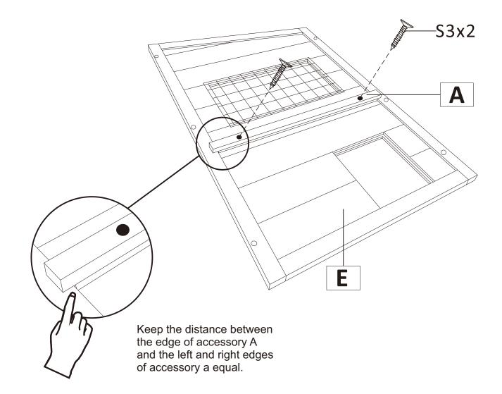
Pay attention to alignment when installing here. A needs to be installed on the back side of E.
