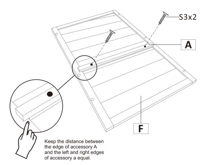
Pay attention to alignment when installing here. A needs to be installed on the back side of F.
