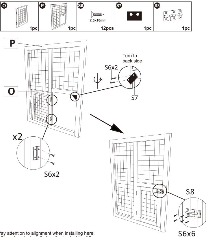
Pay attention to alignment when installing here. S7 needs to be installed on the back side of P to prevent door O from extending excessively.
