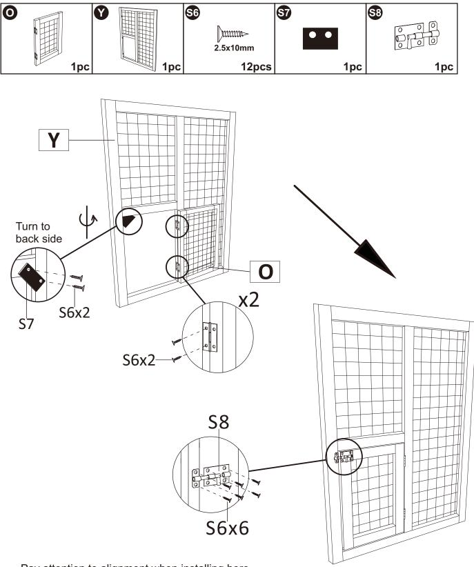
Pay attention to alignment when installing here. S7 needs to be installed on the back side of Y to prevent door O from extending excessively.
