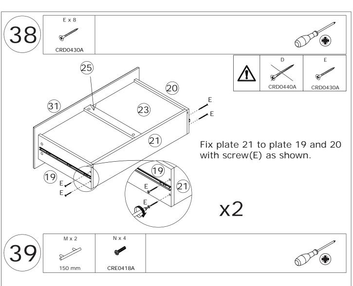
Fix handle(M) with screw(N) as shown.
