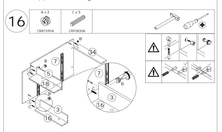
Insert wooden dowel(C) into plate 5,18,3,16 and 34 at first, attach to plate 7 as shown.
