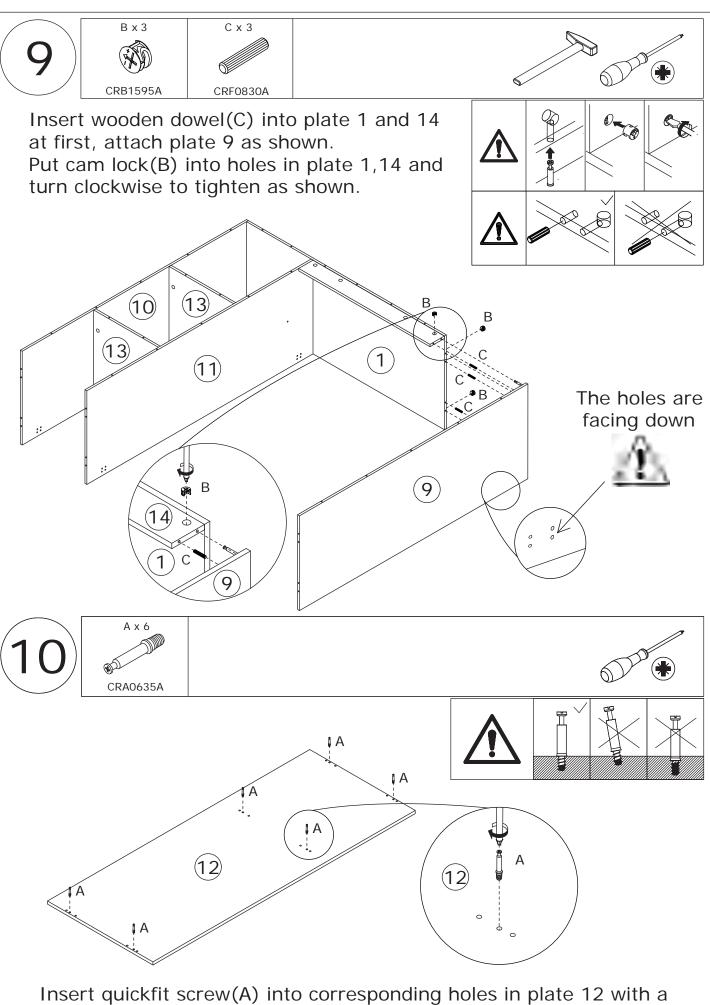
Insert quickfit screw(A) into corresponding holes in plate 12 with a screwdriver as shown. Please pay attention to the holes where the accessories are inserted.
