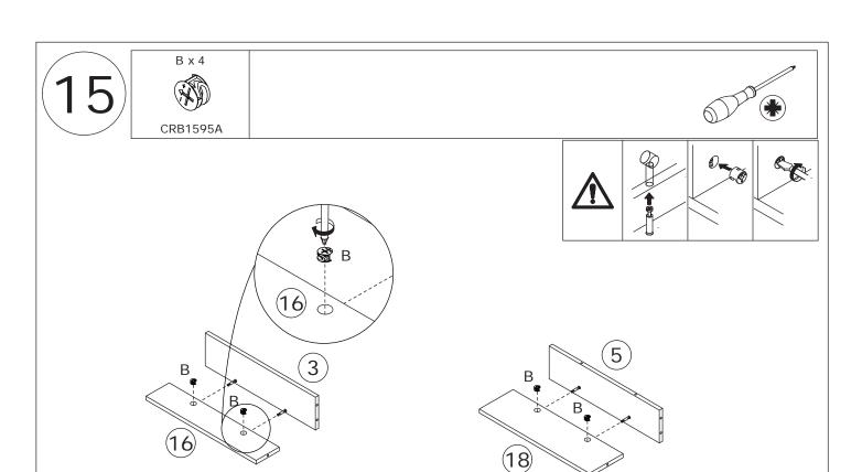
Attach plate 3 to plate 16, plate 5 to plate 18, then turn cam lock(B) clockwise to tighten as shown.
