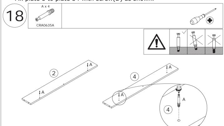
Insert quickfit screw(A) into plate 2 and 4 with a screwdriver as shown.
