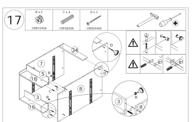
Insert wooden dowel(C) into plate 5,18,3 and 16 at first, attach to plate 8 as shown. Put cam lock(B) into holes in plate 3,5 and turn clockwise to tighten as shown.
