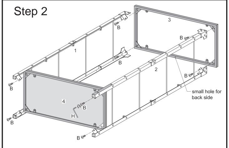
Position the side frames (1,2) and top frame (3) with the small hole toward the floor. Use wrench (H), and bolt (B) to secure the top frame (3) to side frames (1,2).
