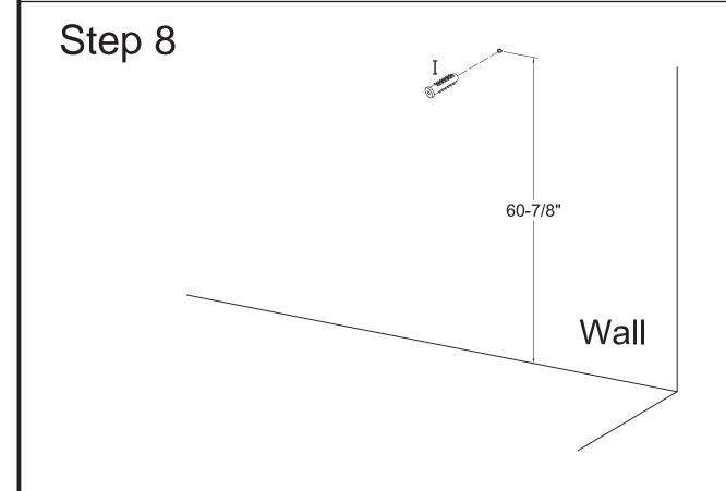
Insert the wall anchor (I) to the wall as per diagram.
