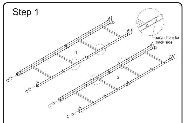
Insert adjustable feet (C) into the side frames (1,2). Please pay attention to the small hole for back side to assemble the cross bar (5) then.
