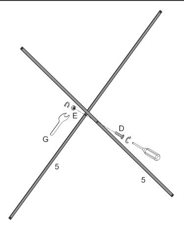
Secure bolt (D), nut (E) by using wrench (G) to the cross bar (5).
