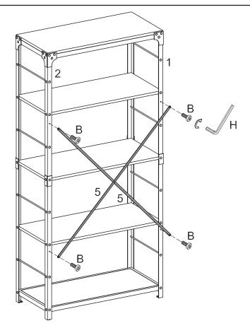
Use wrench (H), bolt (B) to secure the cross bar (5) to back of the side frame (1,2).
