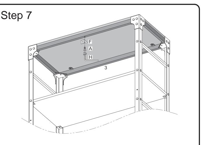
Use wrench (H), bolt (A) to secure the L shape bracket (F) to the top frame (3).
