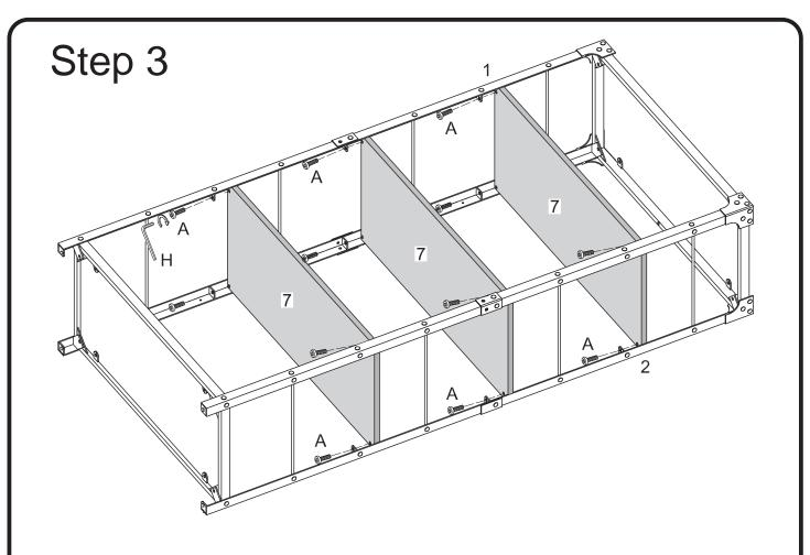
Use wrench (H), bolt (A) to secure the shelf (7) to the side frame (1,2).
