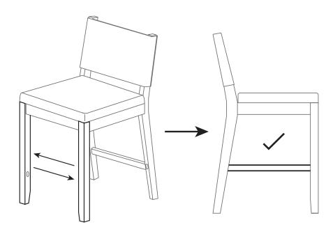
Carefully flip the stool over on a flat surface and make sure the legs are touching the ground evenly before tightening everything to 100%.
