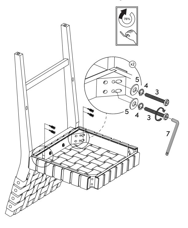
Let's secure those Front Legs (C) & (D) in place using the 1/4 inch x 60mm Hex Button Head Bolt (2), 1/4 inch Lock Washer (4), and 1/4 inch Flat Washer (5).
