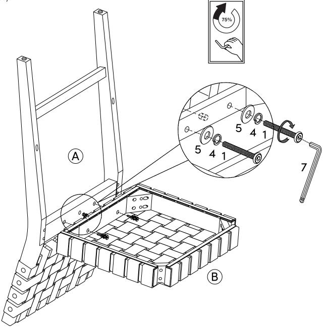
Safety first, then comfort: let's make sure your stool is is sturdy! Secure the Seat Frame (B) using the 1/4 inch x 40mm Hex Button Head Bolt (3), 1/4 inch Lock Washer (4), and 1/4 inch Flat Washer (5).
