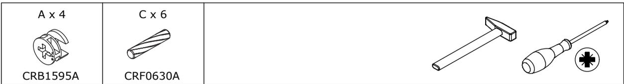
As shown in the figure, use the wooden dowel (C) to connect Panel 12 to the assembled unit, and then insert the eccentric wheel (A) and tighten it by rotating it clockwise.
