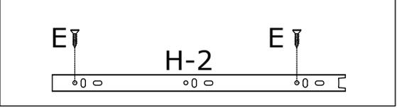
As shown in the figure, use the screw (E) to fix the sliding rail H (H-2) to Panel 2 and 6.
