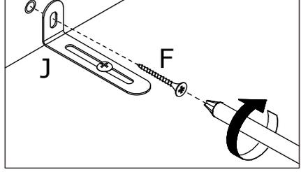
As shown in the figure, install the anti-tipping device.
