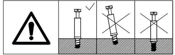
As shown in the figure, screw the self-tapping rod (B) into Panel 12.
