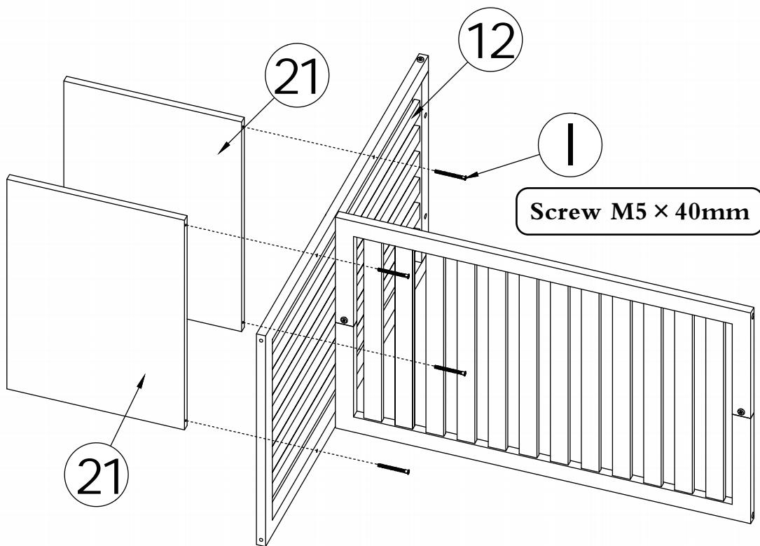
EN-During the assembly, please first half-tighten all the screws into the holes.
