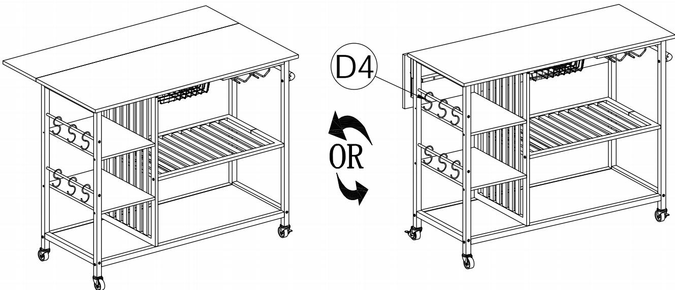
EN-During the assembly, please first half-tighten all the screws into the holes.
