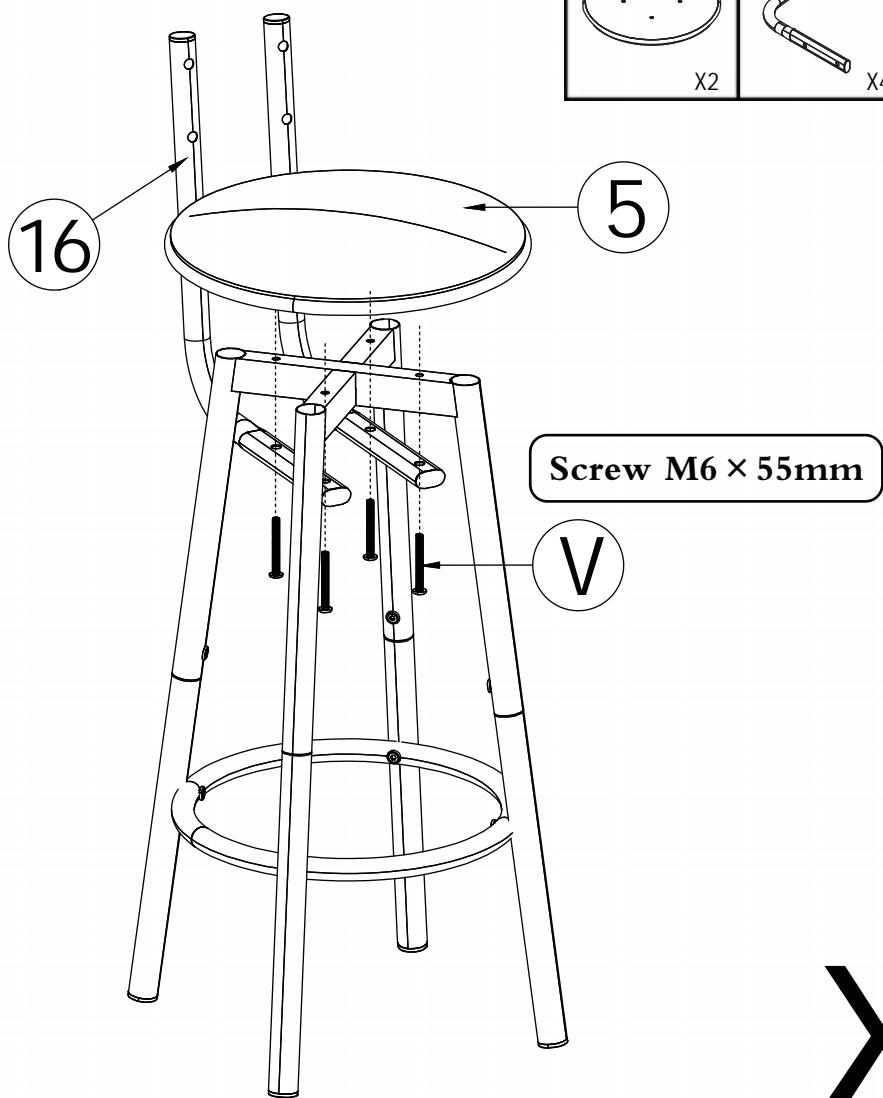
EN-During the assembly, please first half-tighten all the screws into the holes.
