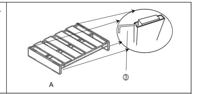
Open the carton and place all the parts onto a clean, non-marring surface., Take out the silders in the four ends of the Seat(A) using Allen Key(③).
