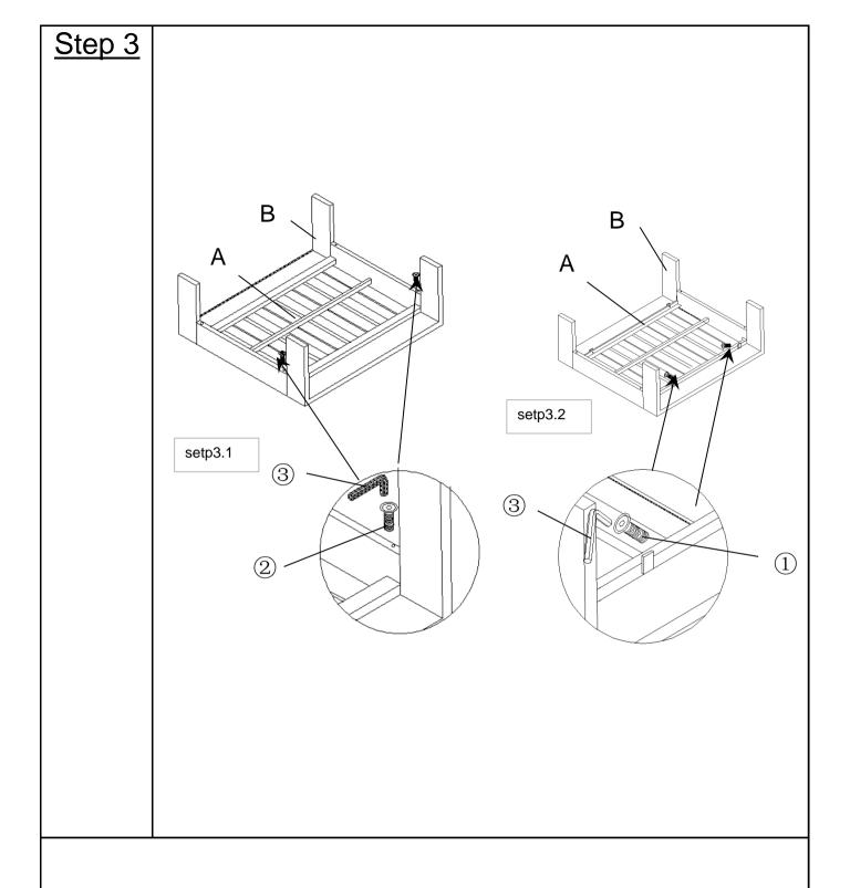
Step3.1:Attach Leg(B) to Seat(A) using Bolts(2) with Allen Key(3) as shown above
