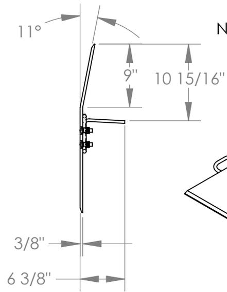
NOTE: BEND OR CROWN IS 11° AND LOCATED 9" FROM EDGE OF DOCKPLATE
