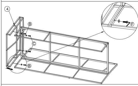
STEP 3: Connect the part from Step 2 and Right Frame (4), tighten Allen Bolt (B), (C) Flat Washer (E) with Allen Key (F).
