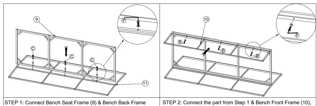
(11), tighten Allen Bolt (C), Flat Washer (E) with Allen Key (F).
