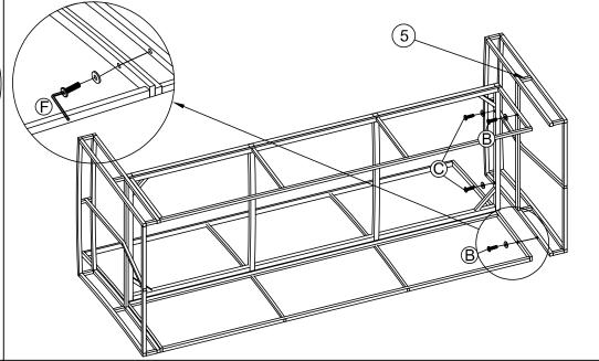
STEP 4: Connect the part from Step 3 and Legt Frame (5), tighten Allen Bolt (B), (C) Flat Washer (E) with Allen Key (F).
