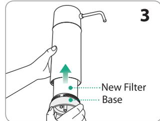
4. Screw the base into the main body.
