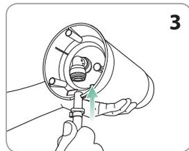
3. Connect the inlet hose to the inlet connection under the base. Then connect the other end of the hose to the faucet diverter.
