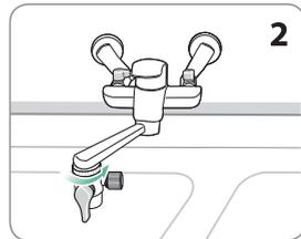
2. Connect the faucet diverter to water faucet by hand tightening using any adapters as needed. If needed, use a wrench (spanner) or pliers, but be careful not to over tighten. Use 2 faucet diverter adapters (included) as needed for proper connection.
