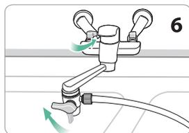
6. Turn on faucet with cold water, turn diverter to open position and check all connections. Let water run through filter for 5 minutes to flush and activate filter.
