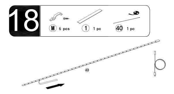
Please tear off the adhesive paper behind the light strip before pasting the light strip to parts#1
