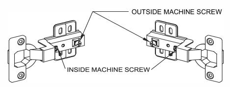
In the event that the door does not align properly, the INSIDE Machine Screws located on the Hinges are for adjusting slightly to the Left or Right. **DO NOT LOOSEN THE OUTSIDE MACHINE SCREW FOR ADJUSTMENT.**
