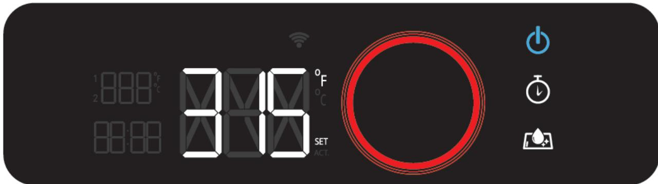
**SET TEMPERATURE** Rotate the control knob clockwise to set a higher temperature. Press the knob and wait until the light ring stops pulsating, indicating target temperature is reached. The display alternates between the current and the desired temperature, "Set" and "Act" flash. Turning counterclockwise decreases the temperature.
