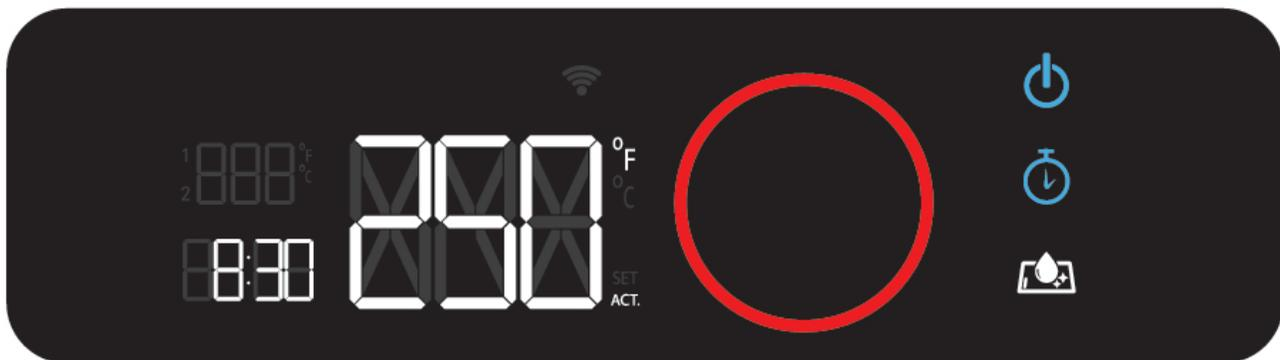
**TIMER & FOOD TEMPERATURE** Pressing the stopwatch symbol activates the timer. The display flashes 00:00. Use the rotary knob to set the time in 30-second increments and confirm by pressing. The LEDs for the food temperature sensors are also located on the left. They show the sensor temperatures as soon as they are connected to the griddle.
