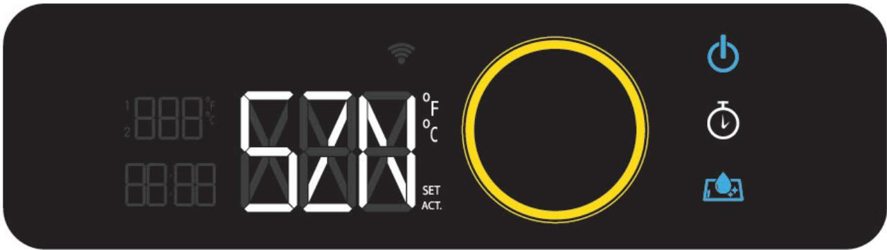
**AUTOSEASON** Coat top surface and walls of griddle with a thin layer of high heat oil. For even better performance, coat the underside of griddle as well. With the lid closed, press the AutoSeason symbol for two seconds until the light ring lights up. The griddle switches off automatically as soon as the program is completed. Repeat this process 3-5 times for optimal results.
