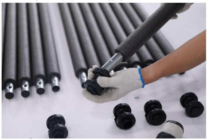
Second, ensure that the two holes are aligned, then secure it with a cone-shaped screw.
