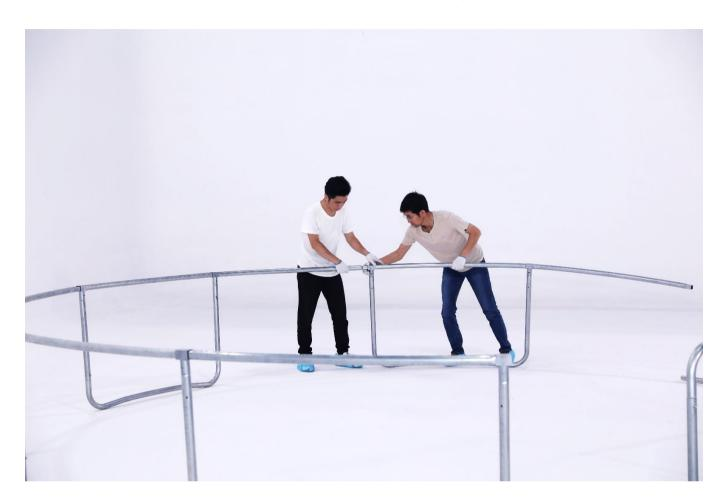
Note: After assembling the frame, temporarily insert the Long Screws (#17) into the locking holes without tightening to maintain the stability of the frame. If the T-shaped Connector (#5) holes are not aligned with the Leg Extension (#7) holes, please rotate the U-Shaped leg tube horizontally at 180 degrees (swap left and right).
