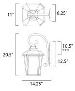
\*height from top of the fixture to center of outlet
