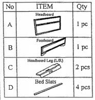
STEP 1: Attach Head Board Leg (C) to Head Board (A) as shown using JCBC BOLT (1) with Spring Washer (2), Flat washer (3) and securing with ALL. KEY (4).
