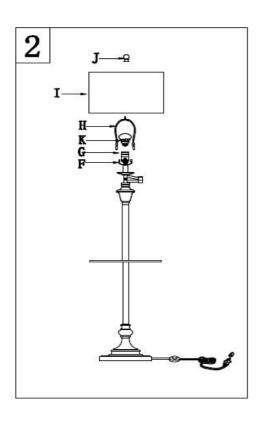
Step 2 Insert the Harp (H) into the Saddle (F). Put the shade(I) on the Harp(H), then tighten the Finial (J) into the Harp (H) Insert the bulb(K) into the socket(G).
