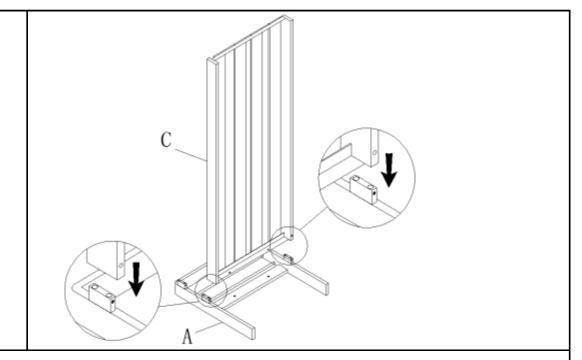
Place the Side Panel(A) with its inside facing up. Insert Seat Panel(C) into the Side Panel(A).
