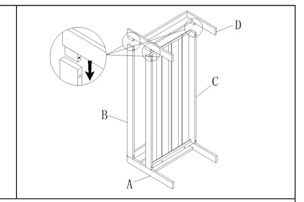
Insert the Leg Support Bar(D) into the Back Support Bar(B) and Seat Panel(C) as shown above.
