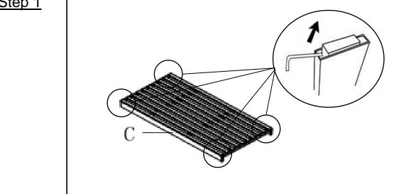
Open the carton and place all the parts onto a clean, non-marring surface. Take out the plastic plug (prevent the alum tube was scratched) in the four ends of the Seat Board(C) using Allen key (2) as shown above.
