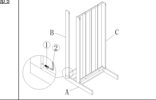
Attach the Back Support Bar(B) to the Side Panel(A) using Bolt(1) with Allen Key(2). **Do not fully tighten Bolt.**
