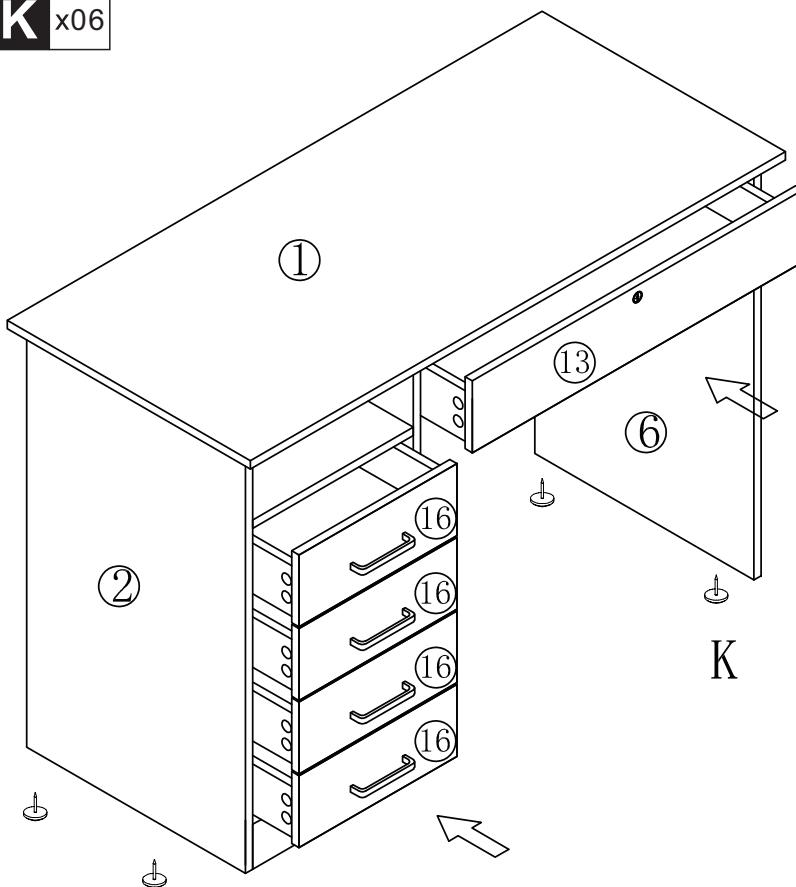
**EN** Be careful to push in the board when the both sides slide way been aligned.
