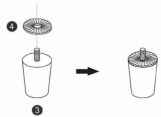
4 Install legs (3) to bottom of assembly
