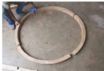
The table framework is fitted together.
