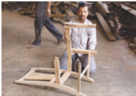
Side rails, stretchers and front legs are assembled.
