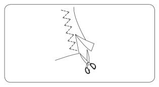
This stitch is used to finish the raw edge on synthetics and other fabrics that tend to pucker. Place your fabric to allow a 1.6 cm (5/8") seam. Trim the seam allowance after sewing. Be careful not to cut the stitches.
