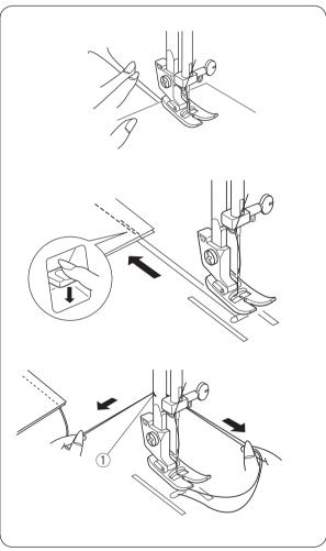
with its edge lining up with a seam guide line on the needle plate.
