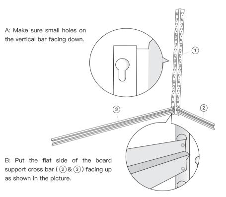
C: Knock on cross bar ( 2&3 ) with rubber hammer until the bar covered the small holes completely.
