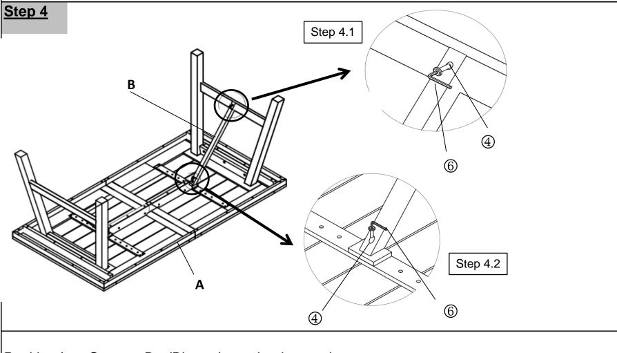
Position Leg Support Bar(B) as shown in picture above.
