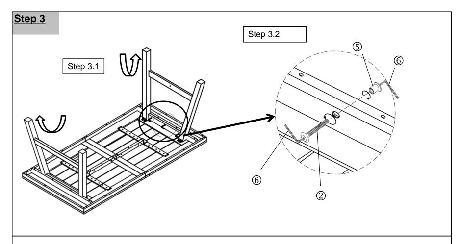
**3.1)** Lift legs upwards and outwards until they are flush with the base of the Table, as shown in the above picture.
