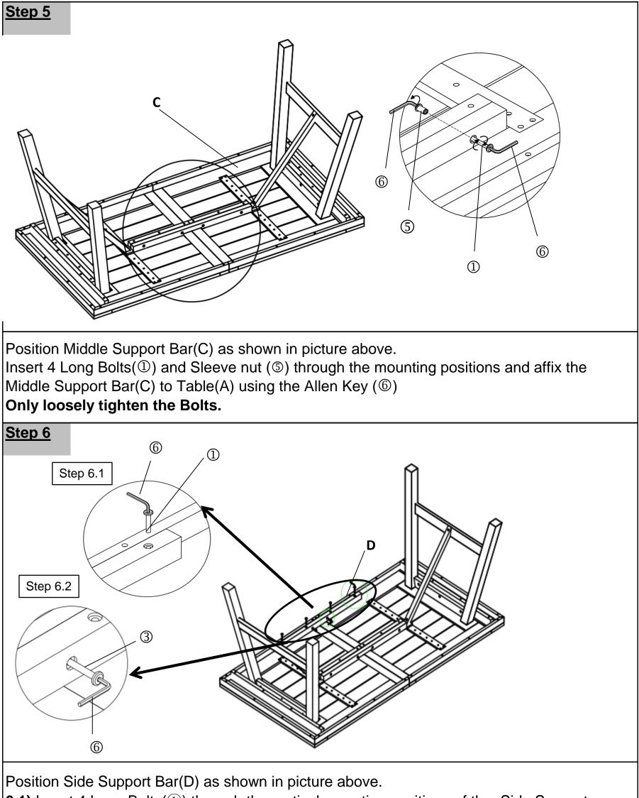
**6.1)** Insert 4 Long Bolts(1) through the vertical mounting positions of the Side Support Bar(D) and affix using Allen Key(6)
