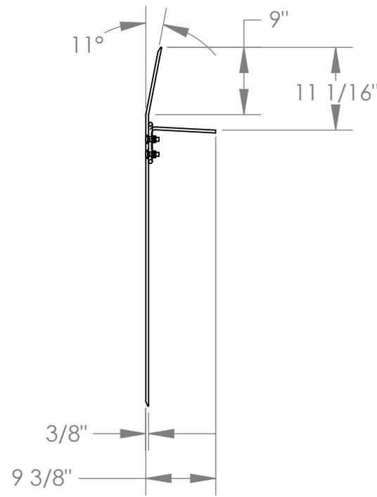
NOTE: BEND OR CROWN IS 11° AND LOCATED 9" FROM EDGE OF DOCKPLATE
