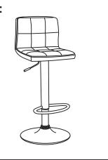
In order to activate the gas hydraulic, it is important that once you have assembled the stool that you raise the lever and bounce your weight up and down on the stool. And then lift your weight off with the lever still raised and the stool should begin to rise.
