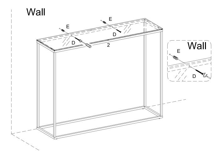
Using Screw (D) attach part (2) into Nut (E) to Wall with Philips head screwdriver as per diagram.
