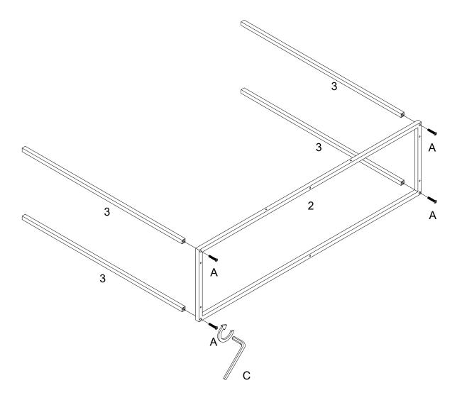
Using Bolts (A) attach part (2) to part (3) with hex key (C) as per diagram. Note: Do not fully tighten all the bolts .
