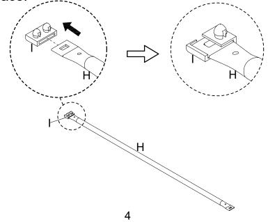
Attach the Slat (H) to assembled rails, put the Slat Connectors (J) & (I) into the correct places and press them down.
