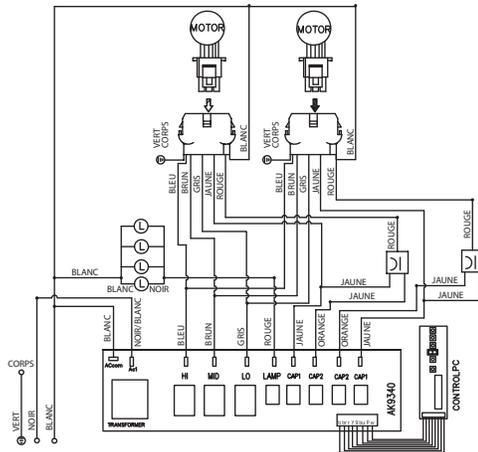
REMARKS:CONDENSER 11+11uF /250VAC 2PCS FIT AC120V 60Hz
