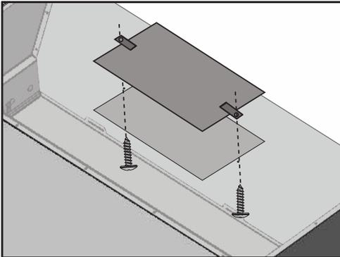
9. Place top rectangular cover plate over opening on top of the liner. NOTE: Make sure the cover plate tabs are on top of the cover plate as shown. From inside the liner, secure plate to top of liner with (2) 3/16 x 3/8 screws.
