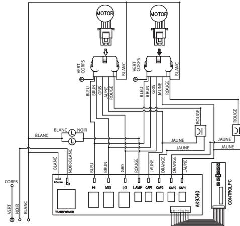
REMARKS:CONDENSER 11+11uF /250VAC 2PCS FIT AC120V 60Hz
