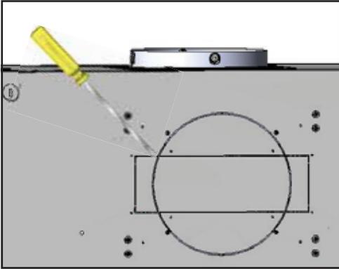
7. Using a flat head screwdriver, remove 8" round or 3 1/4"x10" rect. knock-out plates at the back of the liner.
