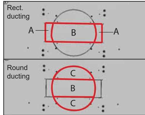
8. Remove knock-outs A and B for rectangular ducting. Remove knock outs B and C for round ducting.
