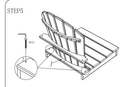
Attach the Back Panel (B) to the Seat Panel (A) with Bolt M6\*45 (M645) by using Allen Wrench .
