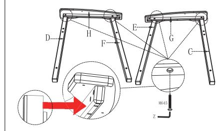
Attach the Right Armrest (G) to the (C&E) and the Left Armrest (H) to the (F&D) with Screws M6\*45 (M645) by using Allen Wrench .
