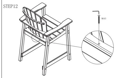
Use the Allen wrench and Screw M6\*45 (M645) to fix the Back Panel Support (J) and Seat Panel Support (I).
