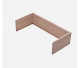
① Position Side Panels (n) and Front Panel (I) as picture shown, secure with Pointed Tail Screw (o).
