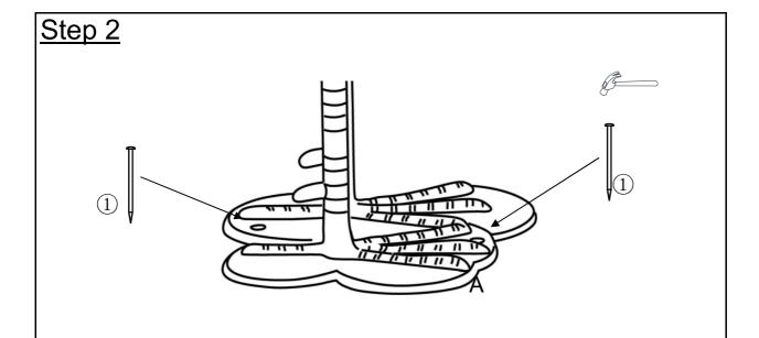
Affix the Crane(A) to the ground by inserting the Stake(1) through the mounting position with Hammer(2).
