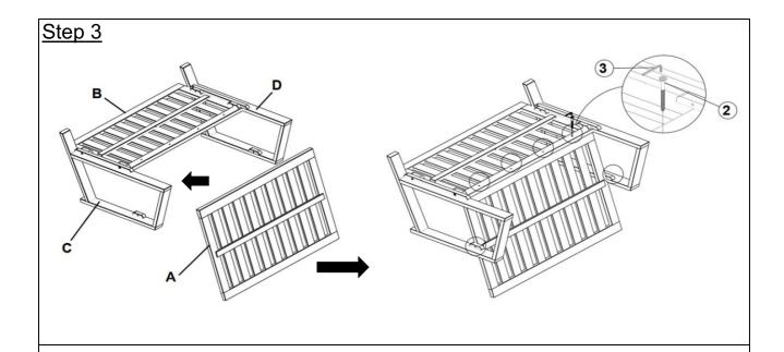
With the help of your adult partner, attach the Backrest Panel (A) to assemble in step 2 Secure the to the Backrest Panel (A) to the Seat Panel (B), Right Arm with Leg (C) and Left Arm with Leg (D) by using Screw(2) and Allen Key (3) as shown above **Do not fully tighten the Screws**
