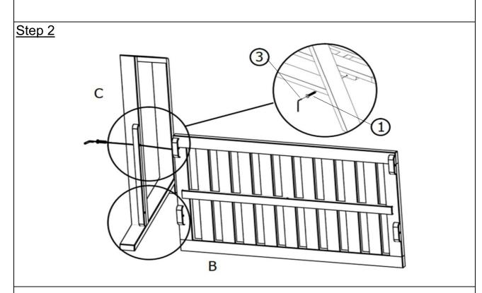
With the help of your adult partner, attach the Right Arrm with Leg (C) to Seat Panel (B) by using Bolt (1) and Allen Key (3) as shown above Repeat the same process with Left Arm with Leg (D)
