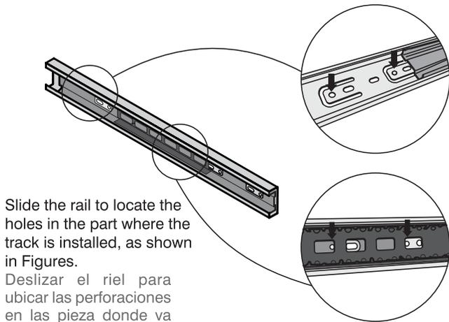
Slide the rail to locate the holes in the part where the track is installed, as shown in Figures.
