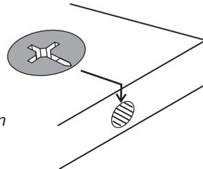
**Do NOT insert the cam studs in the edge holes**
