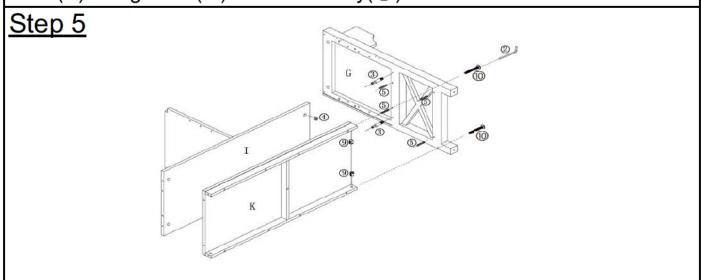
Attach Shelf(I) and Bottom Panel(K) to Dowel(⑤) and Cam Bolt(③) on Right Side Panel(G), insert Cam Lock(④) into Shelf (I) with Screwdriver(⑭), insert Nut(⑨) into Bottom Panel(K) using Bolt(⑩) with Allen Key(②) as shown.
