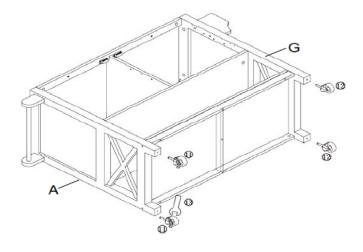
Attach Wheel with brake(1) and Wheel(2) to the Left Side Panel(A) and Right Side Panel(G) with Wrench(3).
