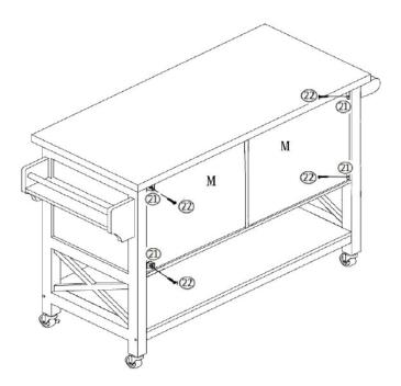
Attach the Buckle(21) to the Back Panel(M) using Screw(22) with Screwdriver(24).
