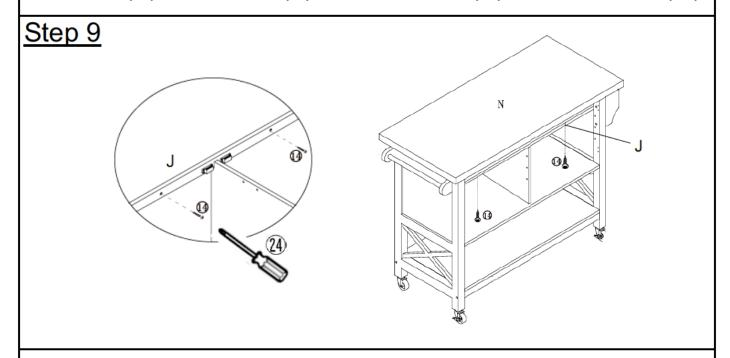
Attach Stretcher(J) to the Top Panel(N) using Screw( $^{\textcircled{4}}$ ) with Screwdriver( $^{\textcircled{2}}$ ) as shown.
