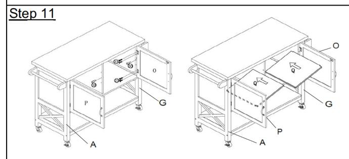
Attach Right Door Panel(O) to Right Side Panel(G) using Screw(3) with Screwdriver(4).
