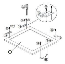
Attach Bracket(1) to Right Door Panel(O) using Screw(1) with Screwdriver(2).
