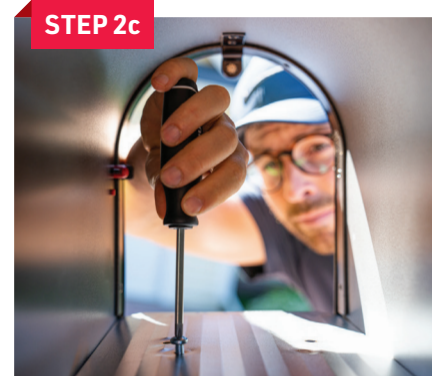
STEP 2c Using the provided hex bolts and nuts, mount the plate to the mailbox using a Phillips screwdriver.
