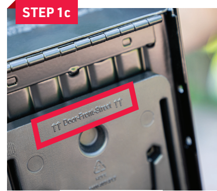
STEP 1c Ensure Door-Front-Street type on bottom of plate is in close alignment with the front of mailbox door. See box modification.
