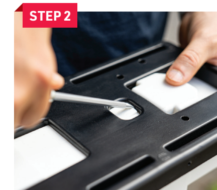
STEP 2 Use a flathead screwdriver to lift the plastic stop behind the catch and slide the mount plate to release.
