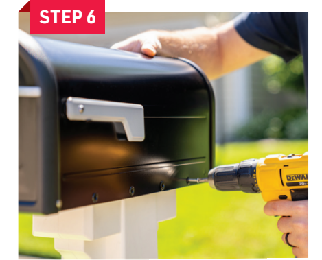
STEP 6 Use drill to drive wood screws through the side holes (4x) to secure to the mounting plate. (Only self-centering solution if mailbox is same width as mount plate.)
