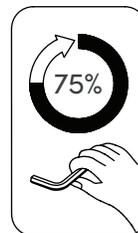
Do NOT overtighten hardware. Tighten only to 75% for now.
