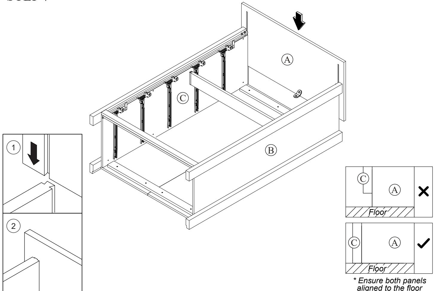
\* Ensure both panels aligned to the floor
