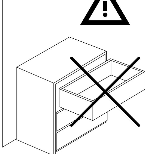
Do not defeat or remove the drawer interlock system. It is important stability and safety system.
