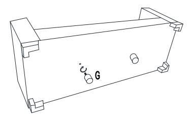
B Hook on the Back Frame (B) to Left Panel (C) & Right Panel (D) properly.
