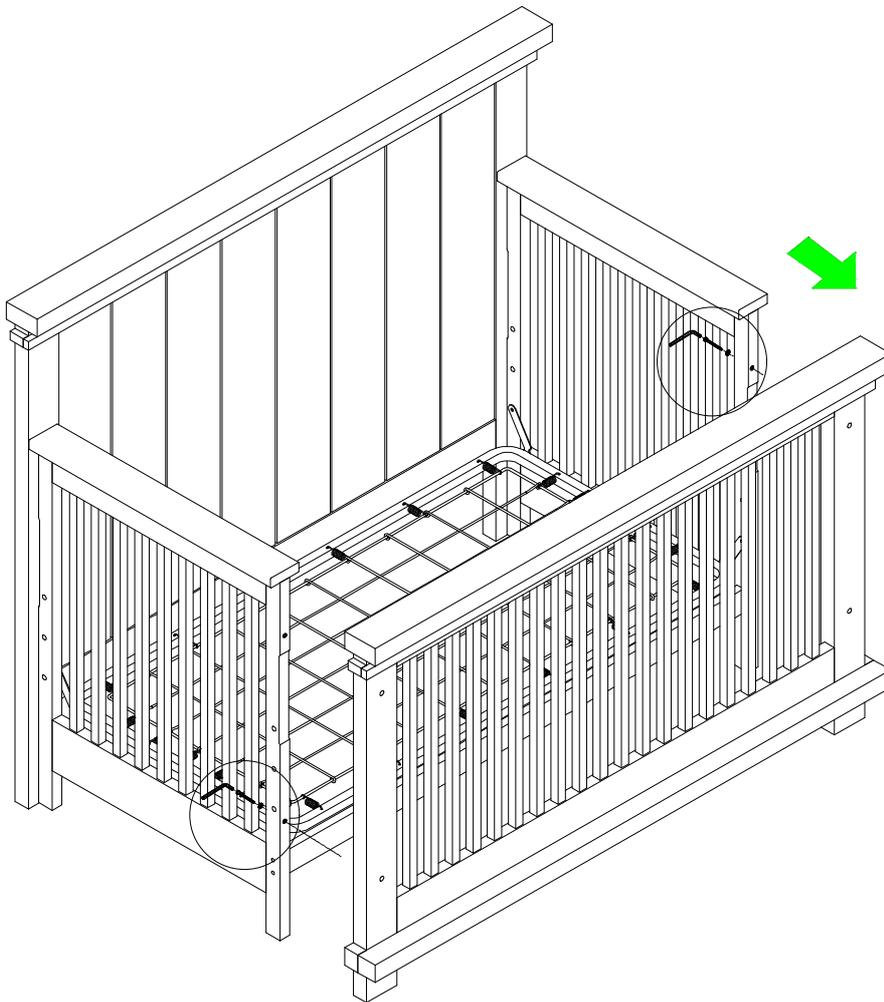
Step 1: Remove Footboard by unscrewing (4pcs) Allen Bolts as shown.
