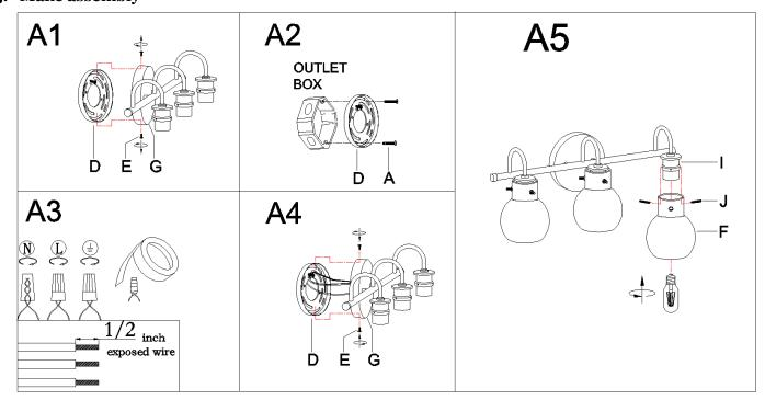
Step A1: Unscrew the studs(E) from the back plate(G) then gently remove the mounting plate (D).
