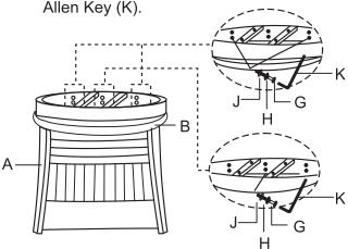
Keep the Backrest (A) and Cushion Seat (B) inverted on a stable raised surface. Attached the Swivel Plate located on the Apron with Swivel Plate (D) to the Cushion Seat (B) using JCBC Screw (F), Flat Washer (J) with Allen Key (K). Turn the Chair right side up.
