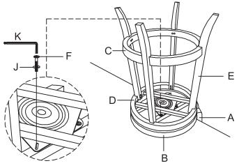
Stand chair up on an even surface and check that it is balanced. If there is a slight wobble, apply downward pressure in the corner where a leg is uneven. Keeping pressure in that corner, tighten all bolts. If balanced, apply downward E pressure evenly in the center and tighten all bolts. Do not over-tighten beyond hole depth.
