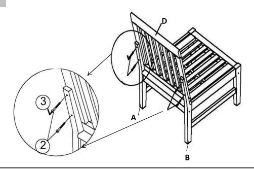
With assistance from your adult partners, turn the Chair right side up Attach Backrest Panel (D) to Right Leg Panel With Pre-installed Levellers (A) and Left Leg Panel With Pre-installed Levellers (B) by using Bolts (2) with Allen Key(3).
