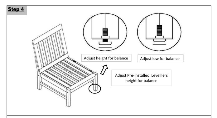
Inspect the Chair and make sure all parts are adequately connected. In a sequential manner, tighten all Bolts and Screws at all joints With assistance from your adult partners, adjust the Levellers to desired height to avoid wobbles
