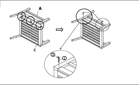
Attach mortise of Left Leg Panel With Pre-installed Levellers (B) to tenon of the Seat Panel (C) Secure by using Screw (1) with Allen Key(3).
