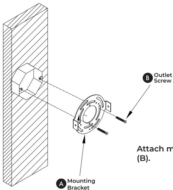
Attach mounting bracket (A) to outlet box with outlet screws (B).
