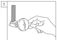
Plug sink drain with cloth to avoid losing small parts. Remove old faucet.
