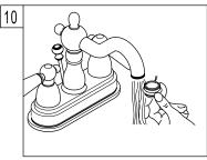
10. Remove the aerator before turning on your new faucet for the first time. This is to prevent any deposits from clogging your aerator. Allow both hot and cold water to run for one minute. Replace aerator.
