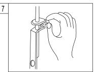
7. With lift rod in position on the faucet, insert lift rod through lift rod strap and secure with the clevis screw.
