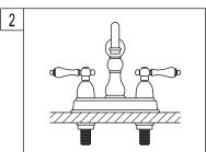
2. Set the faucet in place, insert the inlet shanks through the sink holes, and press down. Assemble the washers and locknuts on the inlet shanks, and then tighten the nuts with
