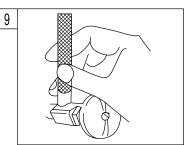
9. Turn on water supply valves and check for leaks, especially at hook-ups to supply lines.
