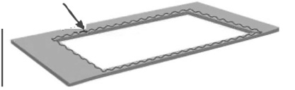
Apply Silicone Sealant After Cleaning The Sink Edge And Countertop
