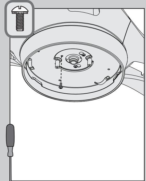
⊗ Insert the third screw, found in the
