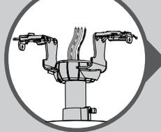
Using an orange wire connector from the ★ hardware bag, connect the 3 grounding wires (green, green/yellow stripe, or bare copper) coming from the ceiling, downrod, and hanging bracket.
