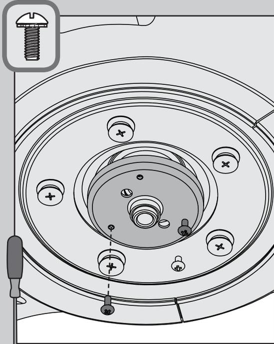
⊗ Screw two housing assembly screws from the
