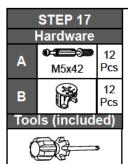
For each of the 3 drawers, assemble the front panel 22 to panels 23 and 24 with bolts A and cam locks B as explained in the Cam Lock Tutorial Page.
