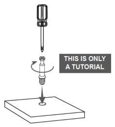
3. Insert the cam lock on the panel with the big hole making sure it goes aligned to receive the bolt's head.
