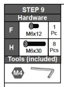
Assemble the shelves 17 to the frames 1 and 2 with screws H from underneath as shown.
