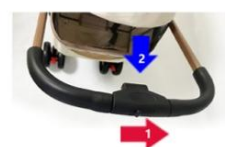
1. Rear bracket of the main frame 2. Pull the buckle to fix the front of the main frame
